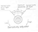
When sensing a delicate and slight color difference such as light yellow on a white paper, warm up the sensor for 30 to 60 minutes prior to the sensitivity adjustment.
