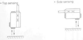
Set the sensitivity adjuster to the min. position. Turn the adjuster clockwise slowly, and reach the point where the sensor turns on in "light" state by a high reflective object. To reach the point where the sensor turns off in "dark" state by a low reflective object. Set the adjuster halfway between these two points for the optimum sensitivity. (Adjuster can be turned approx, eight times )
